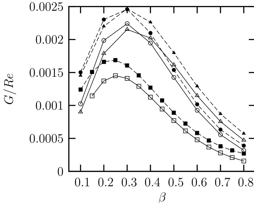
Objective function  $G/Re$ : effect of  $x_{in}$  and  $\beta$  and norm choice (PEN vs. FEN) for  $M = 3$ ,  $T_w/T_{ad} = 1$ ,  $x_{out} = 1.0$ .  $\square$ ,  $x_{in} = 0.0$ ;  $\circ$ ,  $x_{in} = 0.2$ ;  $\Delta$ ,  $x_{in} = 0.4$ .
