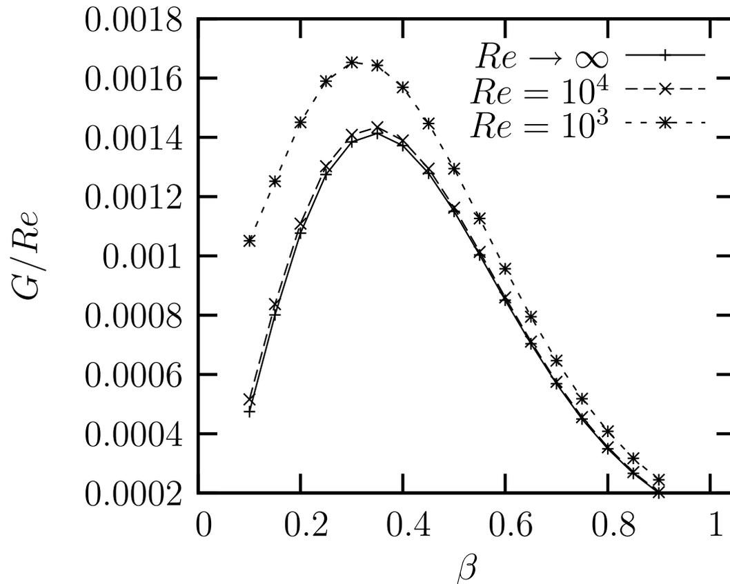
Objective function  $G/Re$ : effect of  $Re$  and  $\beta$  for  $M = 3$ ,  $T_w/T_{ad} = 1$ ,  $x_{in} = 0$   $x_{out} = 1.0$ , FEN.
