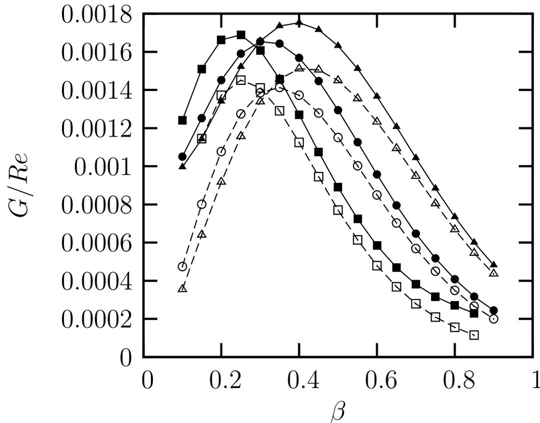
Objective function  $G/Re$ : effect of  $\beta$ ,  $T_w/T_{ad}$  and norm choice (PEN vs. FEN) for  $M = 3$ ,  $Re = 10^3$ ,  $x_{in} = 0$ ,  $x_{out} = 1.0$ .  $\square$ ,  $T_w/T_{ad} = 1.00$ ;  $\circ$ ,  $T_w/T_{ad} = 0.50$ ;  $\triangle$ ,  $T_w/T_{ad} = 0.25$ .
