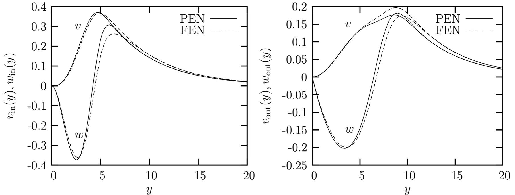
Inlet and outlet profiles: effect of norm choice (PEN vs. FEN) for  $M = 3.0$ ,  $Re = 10^3$ ,  $x_{in} = 0.4$ ,  $x_{out} = 1.0$  and  $\beta = 0.1$ .
