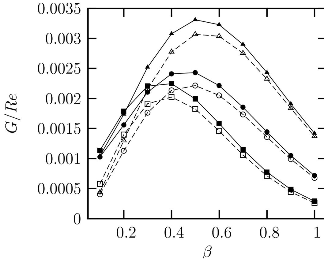
Objective function  $G/Re$ : effect of  $\beta$ ,  $T_w/T_{ad}$  and norm choice (PEN vs. FEN) for  $M = 1.5$ ,  $Re = 10^3$ ,  $x_{in} = 0$   $x_{out} = 1.0$ .  $\square$ ,  $T_w/T_{ad} = 1.00$ ;  $\circ$ ,  $T_w/T_{ad} = 0.50$ ;  $\triangle$ ,  $T_w/T_{ad} = 0.25$ .
