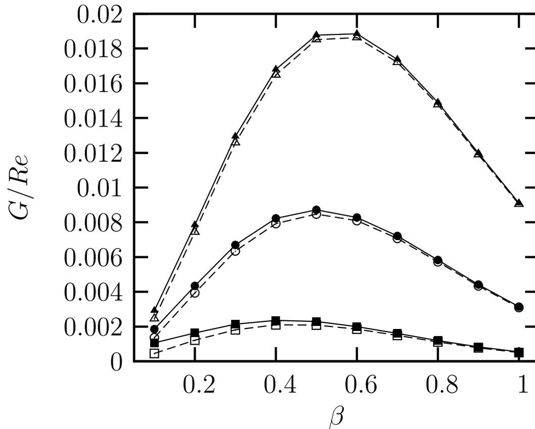
Objective function  $G/Re$ : effect of  $\beta$ ,  $T_w/T_{ad}$  and norm choice (PEN vs. FEN) for  $M = 0.5$ ,  $Re = 10^3$ ,  $x_{in} = 0$   $x_{out} = 1.0$ .  $\square$ ,  $T_w/T_{ad} = 1.00$ ;  $\circ$ ,  $T_w/T_{ad} = 0.50$ ;  $\Delta$ ,  $T_w/T_{ad} = 0.25$ .
