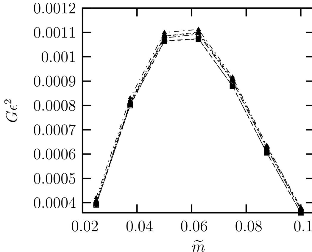
Objective function  $G\epsilon^2$ : effect of  $\epsilon$ , energy norm (PEN vs. FEN) and  $\tilde{m} = m\epsilon$  for  $\theta_{\text{in}} = 2.0$  deg,  $\theta_{\text{out}} = 5.0$  deg,  $\theta_{\text{ref}} = 30.0$  deg,  $T_w/T_{\text{ad}} = 0.5$ .  $\square$ ,  $\epsilon = 1 \cdot 10^{-3}$ ;  $\circ$ ,  $\epsilon = 2 \cdot 10^{-3}$ ;  $\triangle$ ,  $\epsilon = 3 \cdot 10^{-3}$ .
