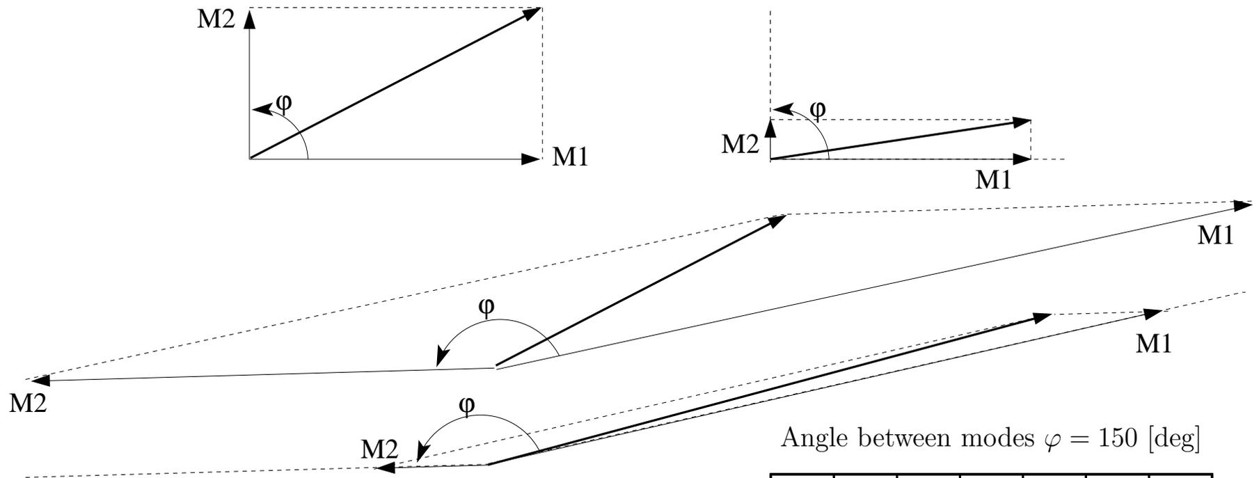
**Non-normality of the operator.** For most flows the linear stability equations are not self-adjoint (the eigenfunctions are not orthogonal)
