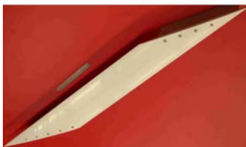
Fig. 1 - 73° swept-wing aluminum model
