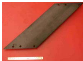
Fig. 2 - 50° swept-wing phenolic model
