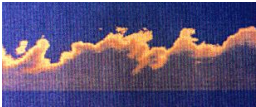
Figure 6.17: Side view images of the instantaneous density field in a Mach 3 turbulent boundary layer. Smith & Smits, 1996.
