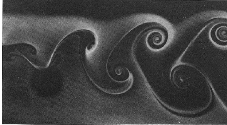
Figure 6.4: Kármán vortex street behind a circular cylinder at Reynolds numbers of 200. From Koopmann.
