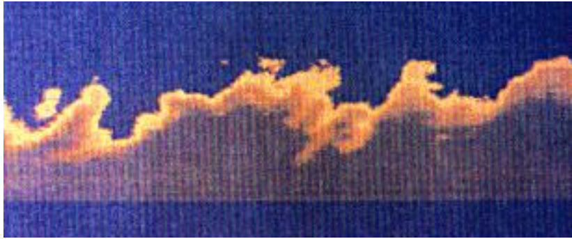
Figure 11.8: Streamwise section of a turbulent boundary layer. Rayleigh scattering image of a turbulent boundary layer at Mach 2.5, by M.W. Smith. Flow is from left to right. Reynolds number based on momentum thickness is about 25,000.
