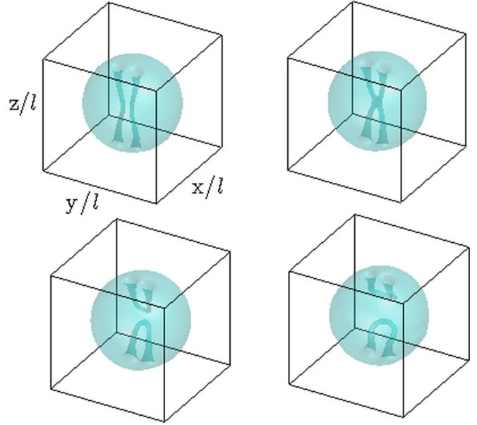
FIG. 1. (Color online) Vortex reconnection in the  $T = 0$  trapped condensate. Density isosurfaces of the dynamics of the initial antiparallel vortex pair, at times  $t\omega = 0$  (top left),  $t\omega = 1.19$  (top right),  $t\omega = 1.80$  (bottom left), and  $t\omega = 2.5$  (bottom right), according to the GPE. The isosurfaces are plotted at 40% of the peak density. The range of the axes is  $-6\ell \leq x, y, z \leq 6\ell$ .
