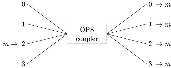
Fig. 1. A  $4 \times 4$  Optical Passive Star (OPS) coupler.
