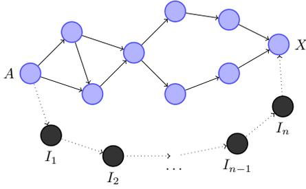
cryptographic operations, the request messages may reach the destination  $X$  faster than in the authorised network. Naturally, this operation can be done within any portion of the network. In the reply, the intruders execute the same operations “back to front”. It is thus an attack of route disruption, since the nodes of the network don’t know the intruders  $I_1, I_2, \dots, I_n$ .
