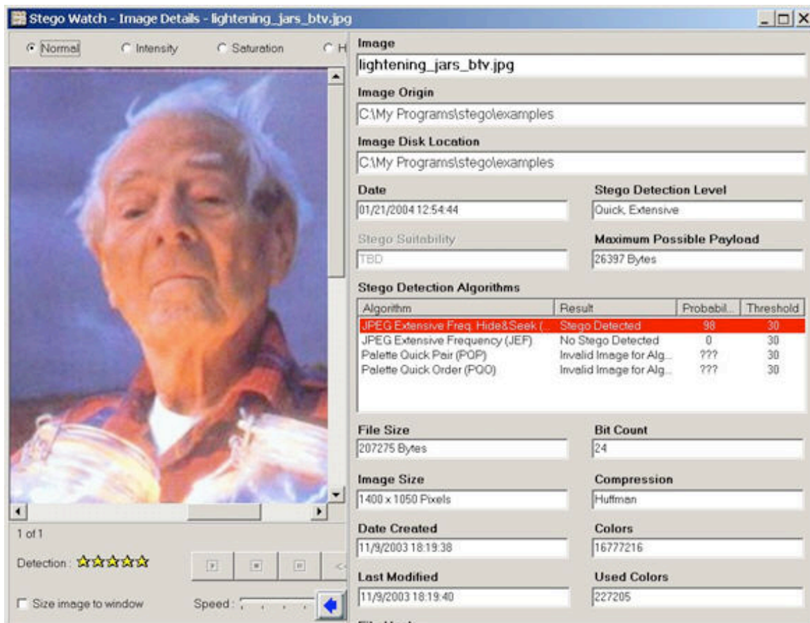
Figure 12. Information from Stego Watch about a JPEG file suspected to be a steganography carrier.
