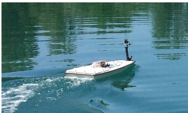
Figure 1: INTCATCH project uses Platypus Lutra boats, about 1m long and 0.5m wide. A camera has been mounted on the front of the ASV.
