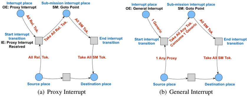
Fig. 5 Types of interrupt implemented in the SPN framework.
