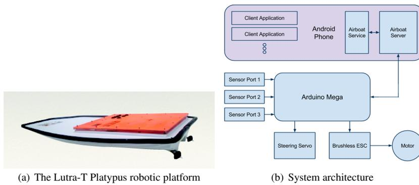
**Fig. 3** A Platypus robotic platform with twin propeller and a diagram of the system architecture
