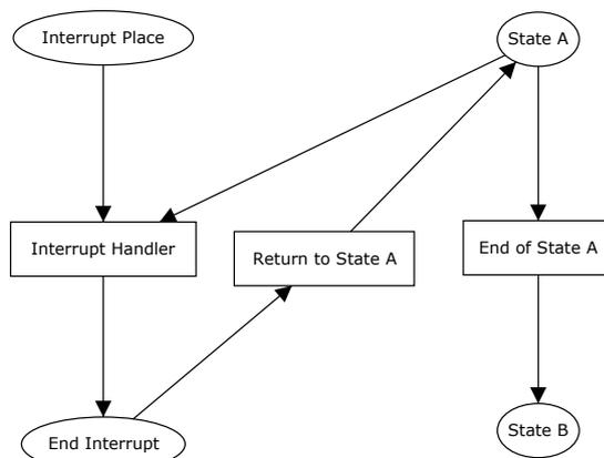
**Fig. 4** Interrupt implementation with Petri Net.
