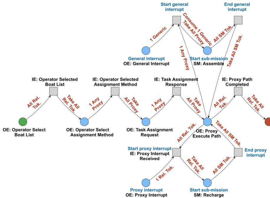
**Fig. 6** The Cooperative Location Visit plan specified in the SPN framework, with both general and proxy interrupts.
