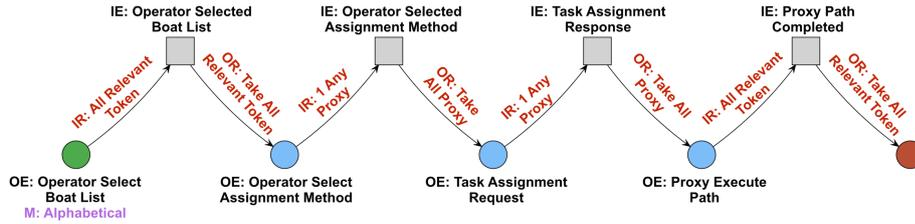
**Fig. 1** SAMI Petri Net “Cooperative Location Visit” plan (without the interrupts). The starting place is colored green and the end place is colored red
