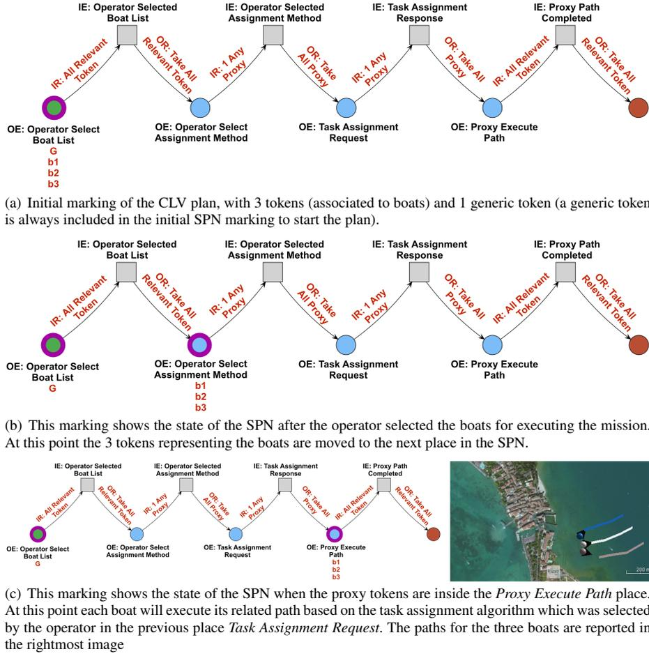
Fig. 2 SAMI Petri Net showing a partial execution of the “CLV” plan (without the interrupts)
