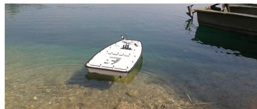
Figure 1: Platypus Lutra equipped with pH, Dissolved oxygen, temperature and electrical conductivity sensors; the computational board is composed by an Arduino Due and a smartphone.
