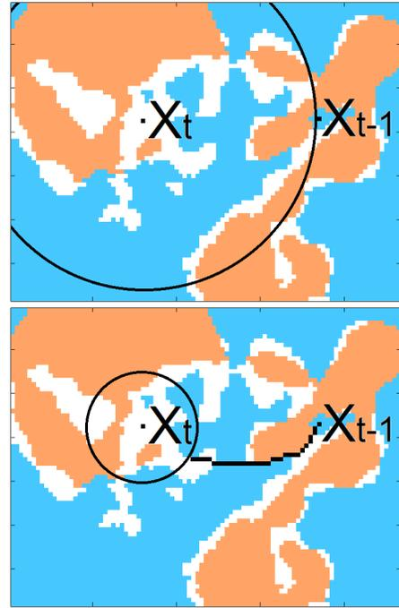
Figure 2: Example of runtime execution of the path selection procedure. The white areas represent location that are still unclassified. The circle represents the area  $A$ . On top the beginning of the procedure and on bottom we can observe the path that has been built after some iterations.
