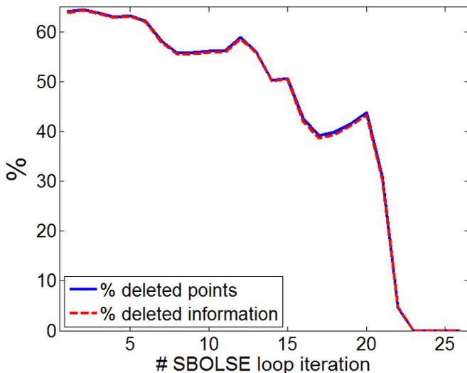
**Figure 7.** Reduction in the number of unclassified points and information after the topological skeletonization, during the execution of the SBOLSE algorithm
