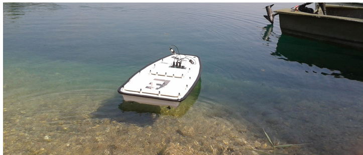
Figure 1: Mobile platform that we used: Platypus Lutra equipped with pH, Dissolved oxygen, temperature and electrical conductivity sensors. The computation is on board and performed by an Arduino Due and a smartphone.
