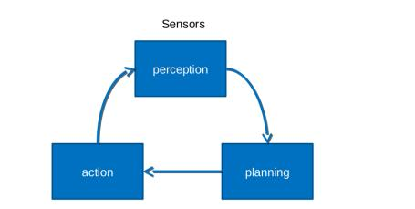
Actuators (motors in mobile robots and manipulators) Learning Data elaboration (e.g. filtering) Make decisions Control architecture
