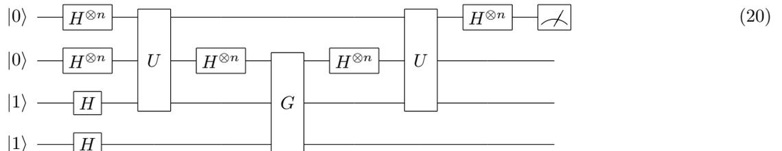
Note that the first two wires on  $n$  qubit quantum wires and the  $G$  gate acts between the second wire and the fourth wire.
