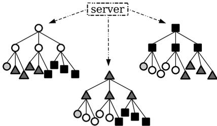
Figure 2.1: Example of a PTree distribution architecture with 13 nodes and 3 stripes, each node appears once in every distribution tree.
