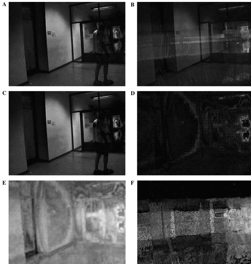
Fig. 14. Activity zones resulting from: (A) MEI over reference frame; (B) MEI over consecutive difference (MMEI); (C) median over reference squared difference (MedReF); (D) median over consecutive squared difference (MedCDif); (E) simple entropy; (F) the proposed approach. The whiter the pixels the higher the activity.
