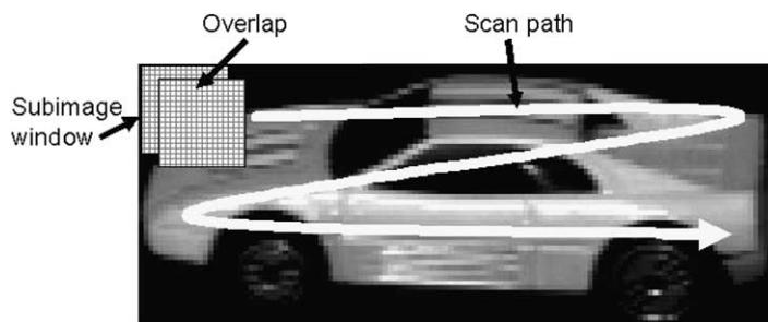
Fig. 1. Sampling scheme to generate the sequence of sub-images.
