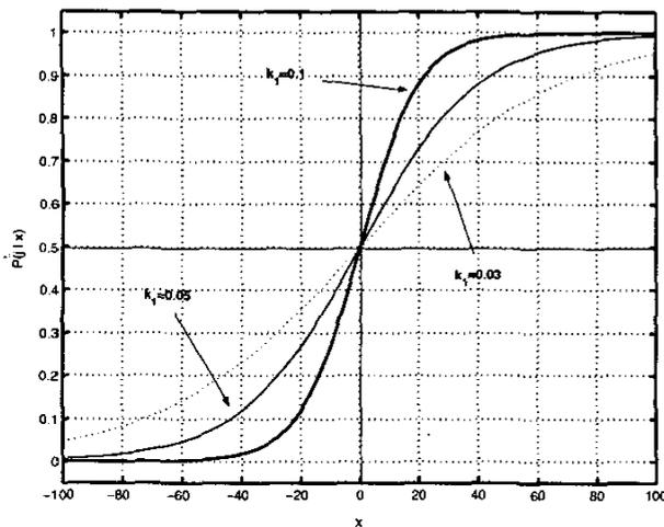
Fig. 4. Sigmoid function used to transform SVM measure into the conditional probability  $P(j|x)$ .  $k$  describes the trend of the sigmoid function.
