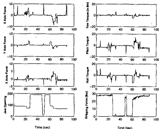
Fig. 5. Force and Torque data during an example of Peg in Hole task. The data are the forces in  $x, y, z$  directions, the torque in  $x, y, z$  directions, the jaw opening and the gripping force.
