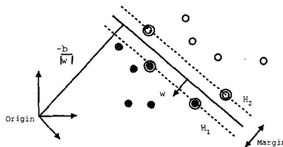
Fig. 3. Separation plane of two example sets (black and white points).
