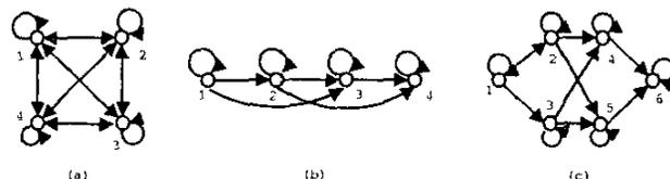
Fig. 2. Three possible types of HMM. (a) A 4-state ergodic model. (b) A 4-state left-right model (c) A 6-state parallel path left-right model.
