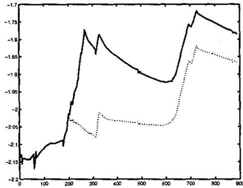
Fig. 8. The *Guard* progress. Solid line represent the *Guard* on real signal while the dotted line represent the *Guard* on modified signal (we have exchanged the real signal with noise in a central interval, from [200, 299]).
