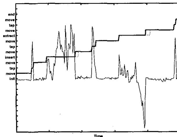
Fig. 7. Peg in Hole segmentation example. Solid line represent the VS segmentation while dotted line represent the VC segmentation, each step indicates a state transition (sub-task).
