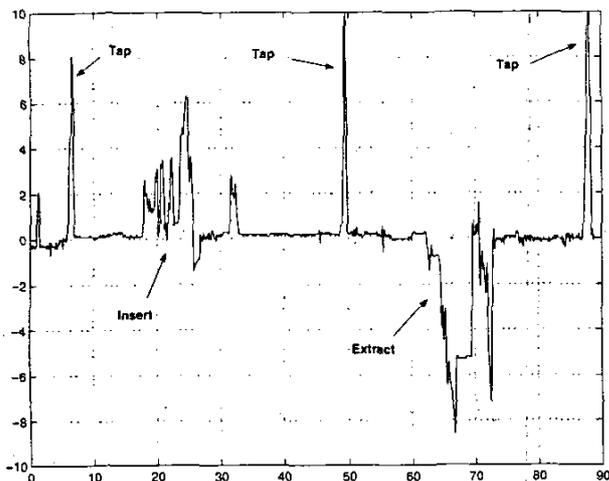
Fig. 6. Force signal in  $x$  direction and the identification of *tap*, *insert* and *extract* sub-task.
