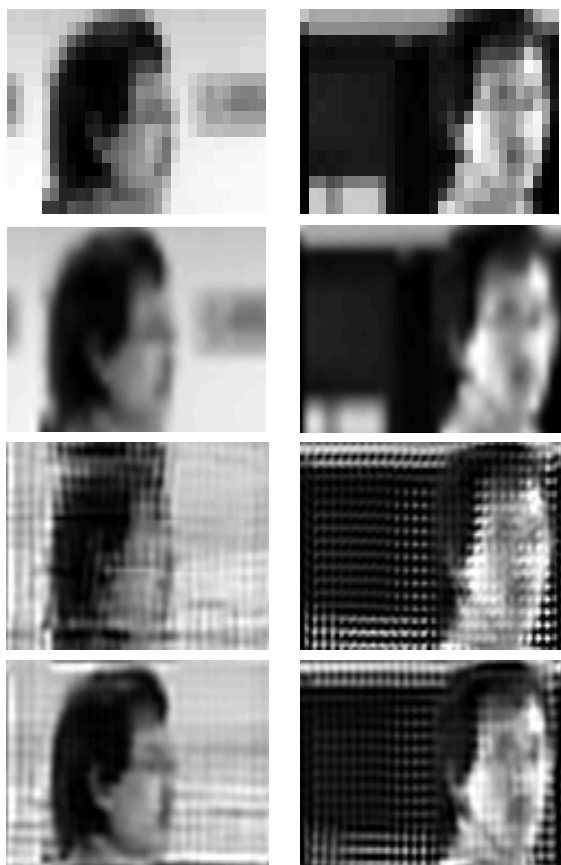
Figure 8: High resolution image estimation results: on the right are the results for the C = 1 cluster, on the left for the C = 3 cluster; from the top: a low resolved image, bi-cubic interpolation, classical Bayesian super-resolution, our approach.
