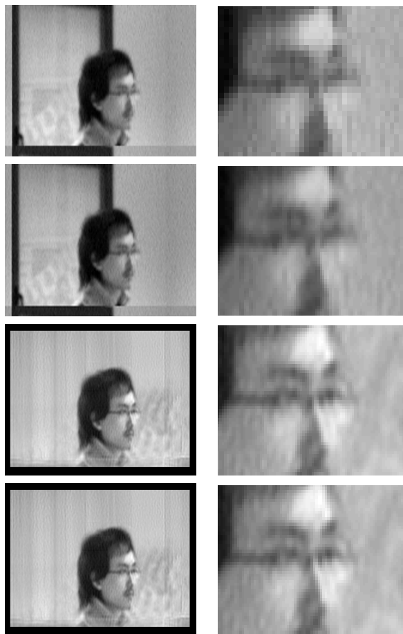
Figure 10: High resolution image estimation results: on the left are the results for the estimated cluster, on the right some enlargements; from the top: a LR image, bi-cubic interpolation, classical Bayesian super-resolution, our approach.
