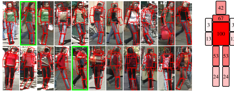
Fig. 3: (Left) Two illustrative lineups in single-shot re-identification from the VIPeR experiments: the leftmost image is the probe and the rest are gallery images sorted by increasing distance from the probe. The correct match is shown with a green outline. (Right) Model of the articulated human figure, with percentages and color intensities proportional to the importance of a part in the VIPeR experiment.
