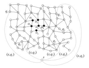
**Fig. 4.** Addition of dummy vertex s to obfuscated multisource graph algorithm, with  $Q = \{q_1, ..., q_5\}$  (gray vertices) and  $O = \{o_1, ..., o_6\}$  (black vertices)
