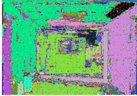
Fig. 11.7. Segmentation of the first indoor sequence using the similarity measure without the HMM states' normalization.
