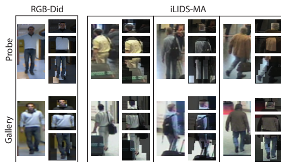
Fig. 1. PTZ re-id datasets: each acquisition of a subject is characterized by four images: the whole-body image (left) and the three zoomed images portraying body parts at high resolution (right). Please note, for each individual we have multiple acquisitions.
