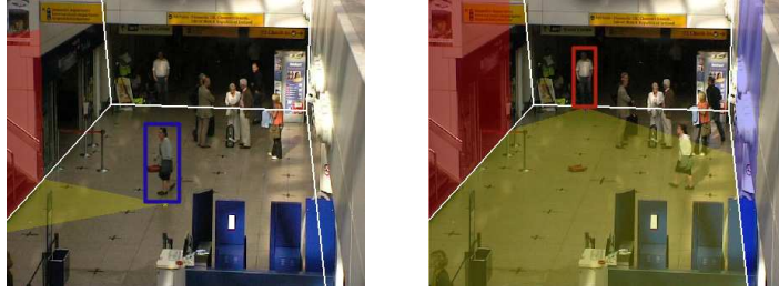
Fig. 3. Two examples of projection of the SVF on the scene main planes. The 3D map permits to suitably model the interactions of the SVF with the scene.
