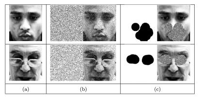
Fig. 6. Example of the masking process on two faces of the database BANCA: (a) original images; (b) random mask and application on the image; (c) mask obtained by deleting the K most important patches (K = 100) and its application on the image.
