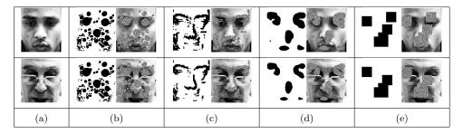
Fig. 7. Example of the masking process on two faces of the BANCA database: (a) original images; (b) Lowe [2004] (SIFT); (c) Salah et al. [2002]; (d) Walther [2006]; (e) Ullman et al. [2002].
